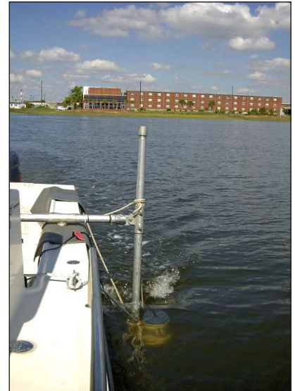
ADCP Data Collection to Quantify River Discharge and Velocity Characteristics of the Charleston Naval Complex
