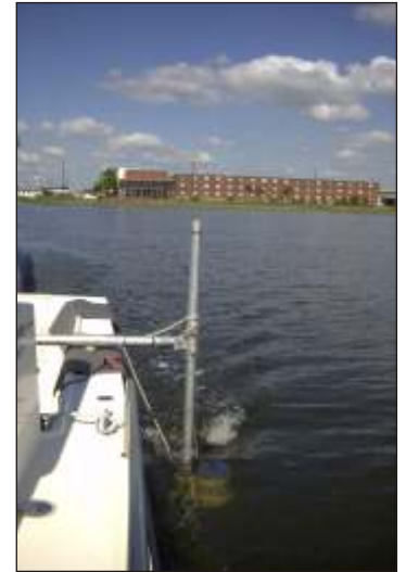
ADCP Data Collection to quantify river discharge and velocity characteristics of the Charleston Naval Complex
